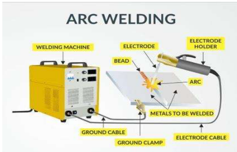
Figures 40: Shielded Metal Arc Welding equipment
